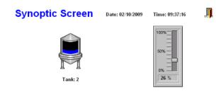
Finished tank selector object during runtime
